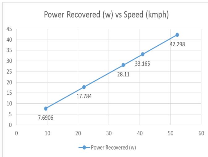
Chart -1: At Constant Braking Load (0.45kg)
