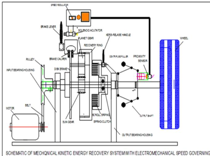
Fig.1 Schematic of mechanical kinetic energy recovery system with electromechanical governing
