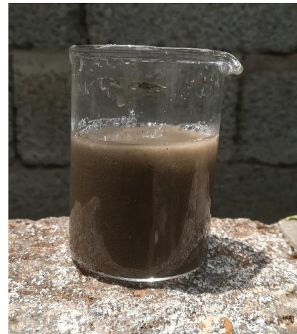
Fig -4: Leachate before passing through liner
