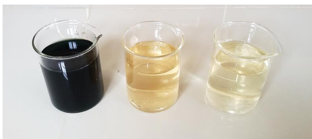
Fig 12 Untreated textile effluent and treated water from macrophytic and root zone system
