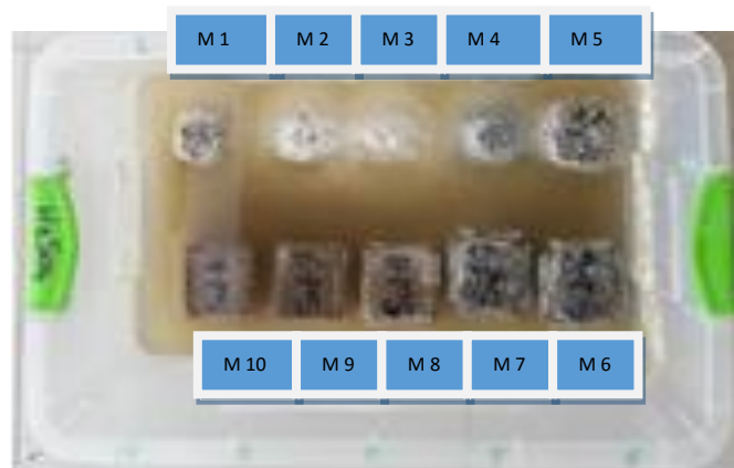
Figure 1: Durability performance of different concrete samples after 90-days exposure to 5% H 2 SO 4 solution.
