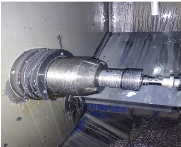
Fig 3. Fixture mount on CNC machine
