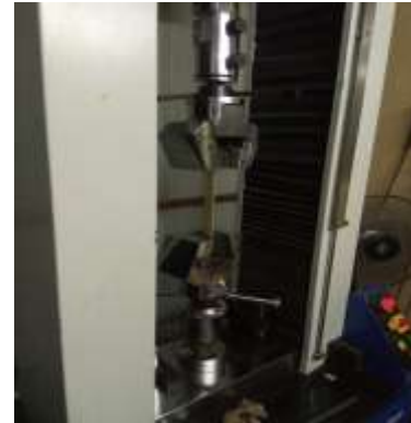
Fig 4.3 Experimental set up for tensile testing
