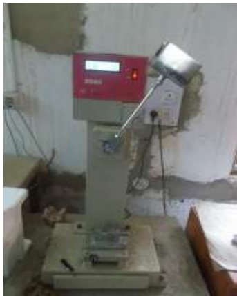
Fig 4.1 Experimental set up for Impact strength test
