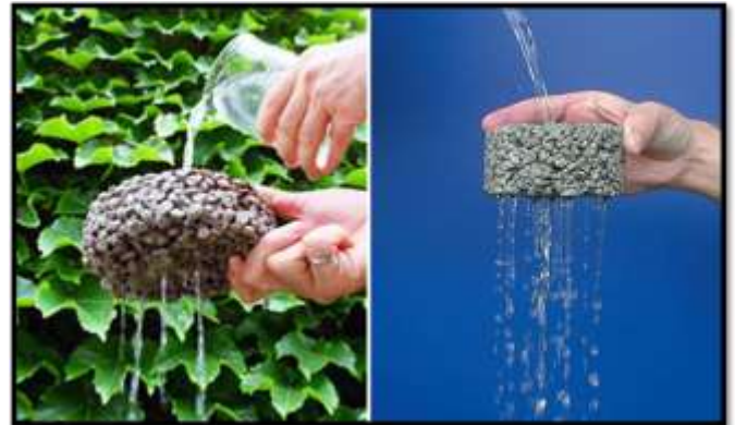
Figure 1.1 Small Model of Porous pavement
