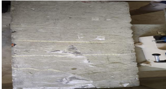
Failure pattern of slab
