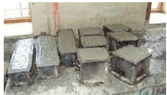
Fig-2: Casting of concrete
