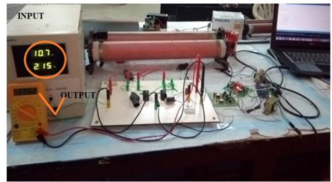
Fig - 42: Experimental results of the Interleaved Boost Converter using DC supply
