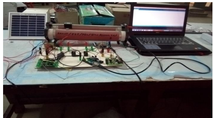
Fig - 44 (a): Experimental results of the Interleaved Boost Converter interface with PV
