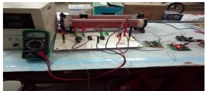
Fig -44 (b): Experimental output of the Interleaved Boost Converter interface with PV
