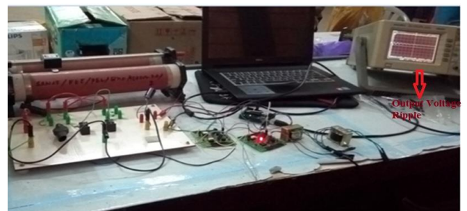
Fig - 43: Experimental waveform of output voltage ripple of the Interleaved Boost Converter using DC supply
