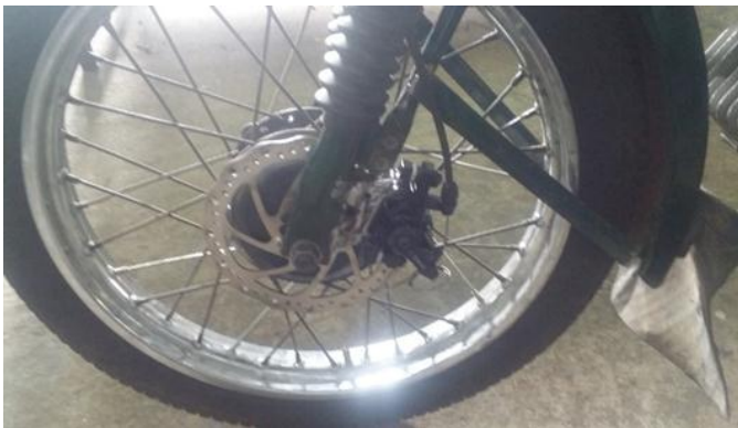
Fig -3: Hub motor assembly
