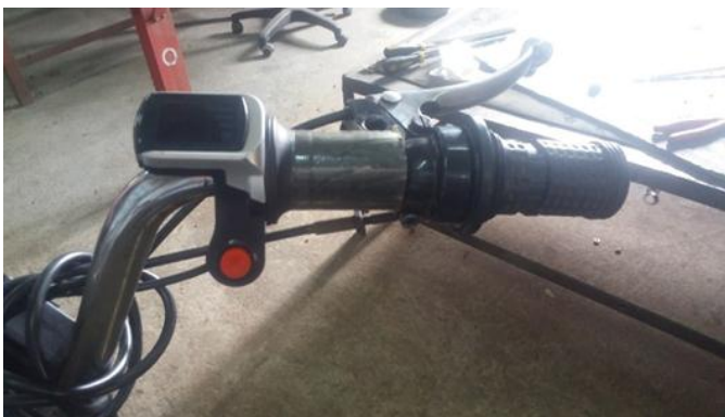
Fig -4 Throttle setup
