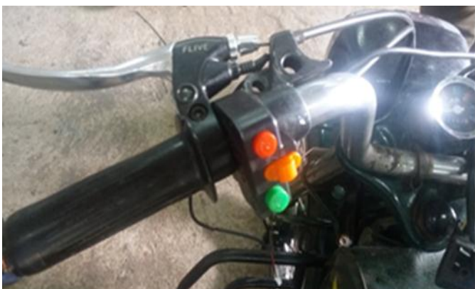
Fig -5: Integrated brake assembly
