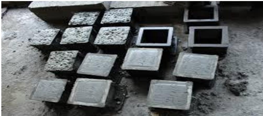
Fig 1. Cube moulds with Concrete
