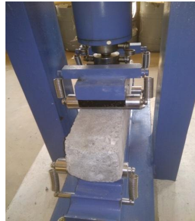
fig 4. Flexural strength testing of prism
