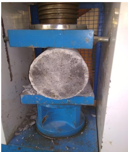
fig 3. Split tensile testing of cylinder
