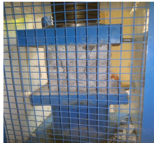
fig 2. Compression testing of cube
