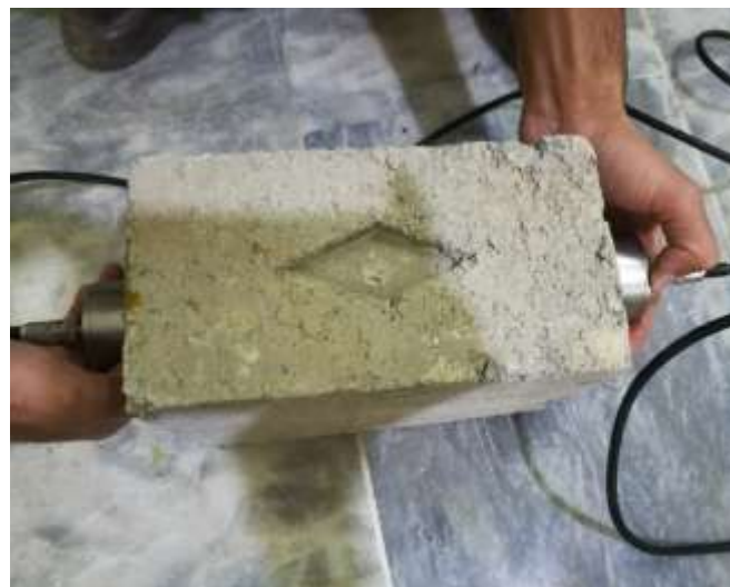
Figure- 8: Testing Boardcrete Specimen Using PUNDIT
