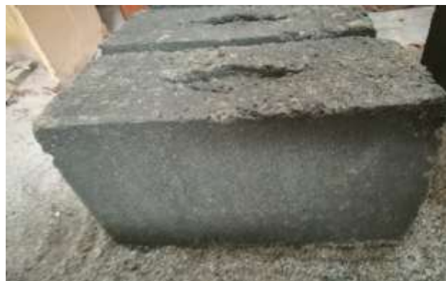
Figure- 4: Boardcrete Specimen after Casting
