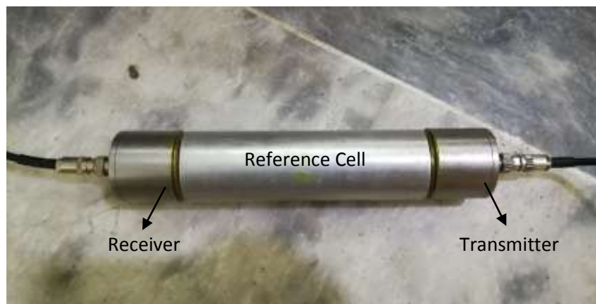
Figure- 6: Calibration of PUNDIT Instrument using Reference Bar
