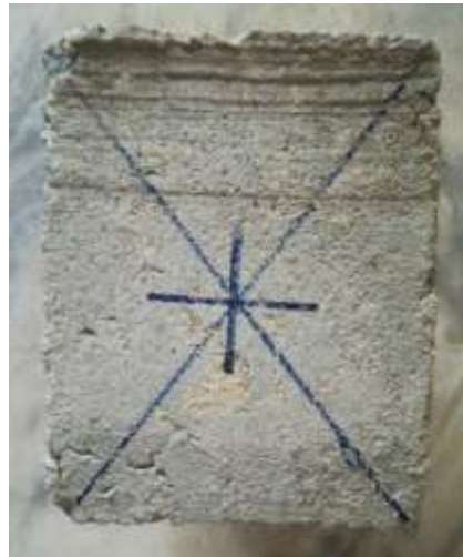
Figure- 7: Marking Boardcrete Face for Proper Positioning
