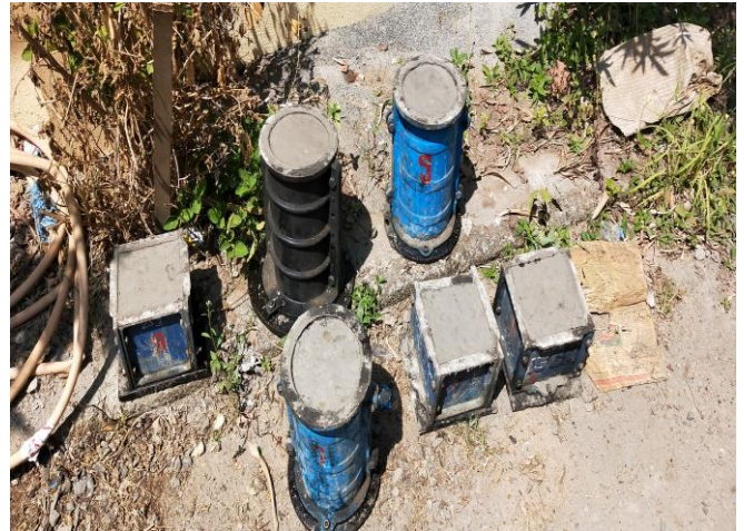
FIG-Specimens Subjected To Sunlight Curing
