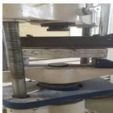
Fig 4.3 Flexural Test machine Flexural Strength = PL/bd 2
