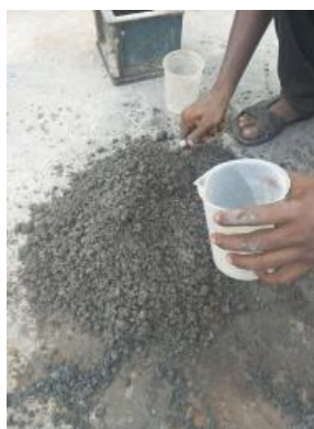
Fig -6.1.2: Water & Polycorboxylate mixing
