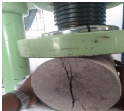
Fig -7.3.2: Split-tensile test of concrete
