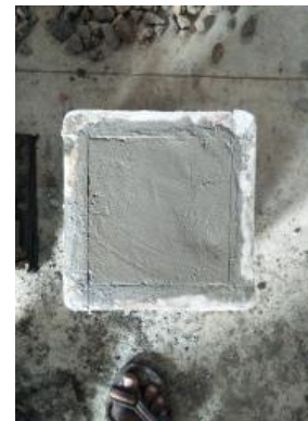
Fig -6.1.2: Coasting concrete in mould
