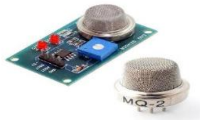
Fig -9: Gas Sensor
