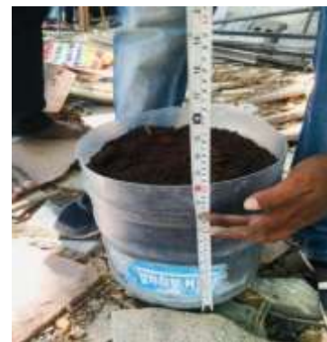
Fig-8 Water Retention Testing Mould
