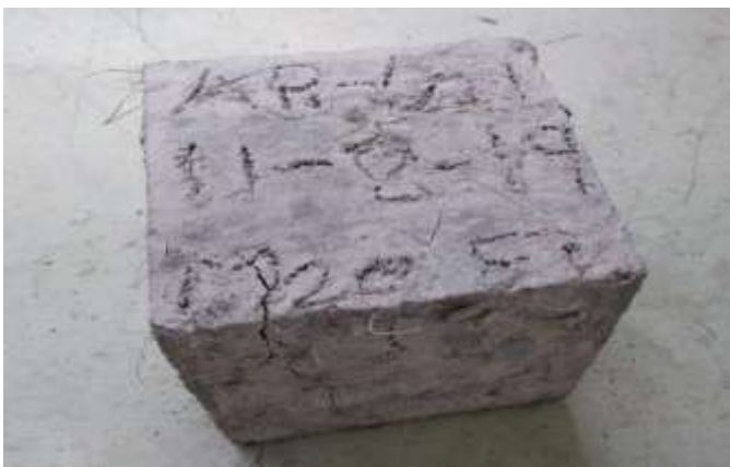
Fig 2: Failure in concrete cube with coconut fiber
