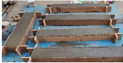
Fig 2 Casting of Beams
