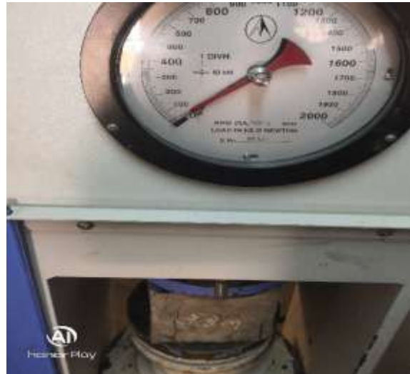
Figure -3 Testing of concrete using CTM
