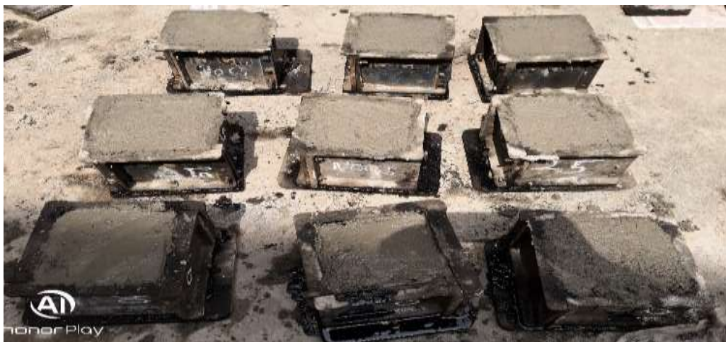
Figure-1 Cellular Lightweight Concrete mould.
