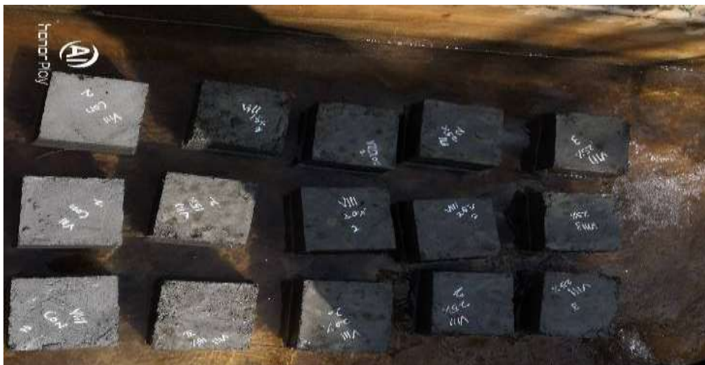
Figure-2: Concrete Cubes Placed for Curing
