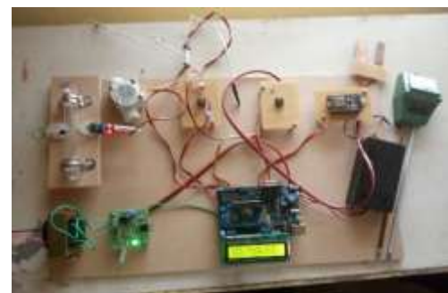
Fig -11: Prototype of the automatic water purifier system
