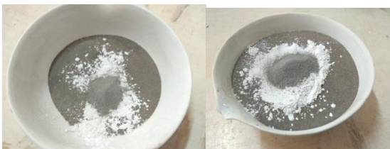
Fig.8 Sample preparation for contaminated soil with WSP and lime
