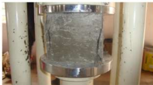
Figure 4.1: Compressive Test on Concrete Cube
