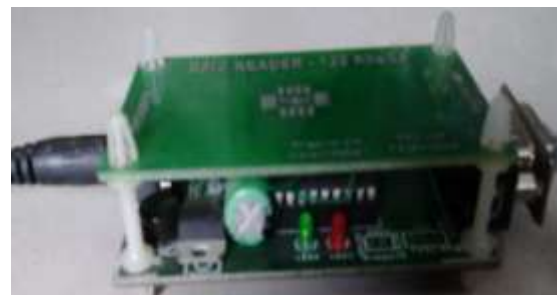
Fig6: RFID Module to be used on the road side
