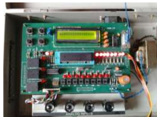
Fig3: Real time embedded system hardware with analog data acquiring
