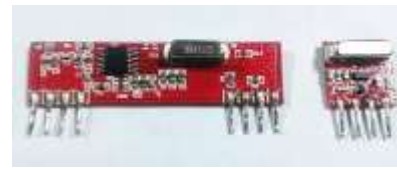
Fig- 3: RF Transmitter & Receiver Module
