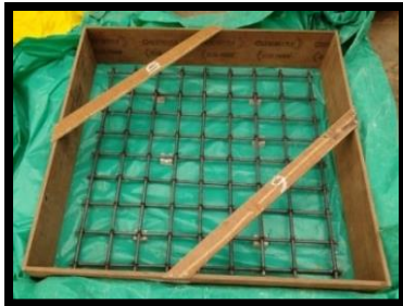
Fig - 1: Reinforcement details of Conventional Slab
