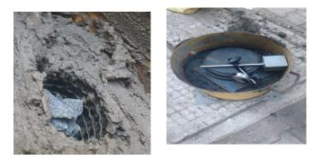
Here, to identify the behaviour of clay soil with encased stone column, firstly the clay soil is excavated using 6cm diameter pipe. Then the geogrid is placed in the hole and is filled with aggregates. Here we have taken square pattern arrangement of stone columns. Load is then applied on the plate. The settlement is noted for every one minute and the graph is drawn between time and settlement for increase in load by 0.5kg.
