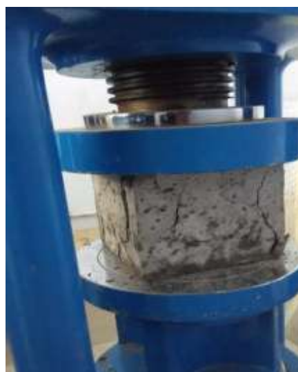
Figure 1.6 Compression strength test for cube
