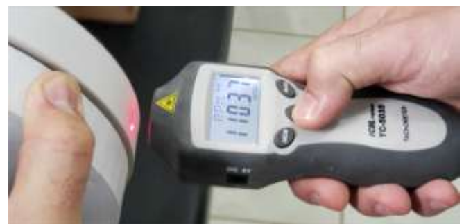
Figure 16 - Tachometer indicating the angular velocity of 110.37 rpm used in the test.
