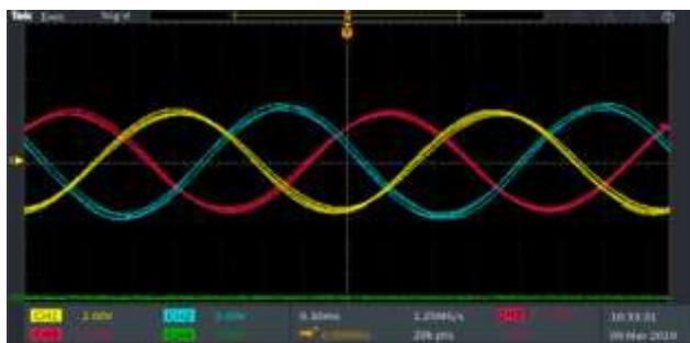
Figure 18 - The three-phase voltage generated in loads of 1 \Omega of 30 W.
