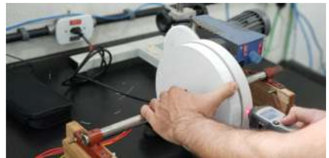
Figure 15 - Controlled bench test of the AFPM Generator.
