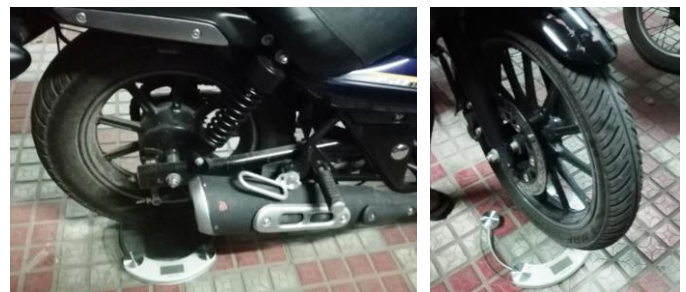
Fig-3.1: Determination of weight shared by front and rear Wheels
