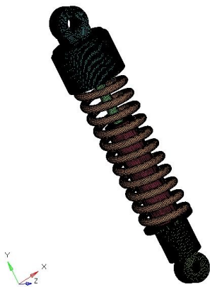
Fig-4.3: Final Mesh Model of Shock Absorber
