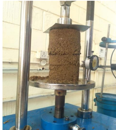
GEOGRID IS PLACED AT CENTRE
