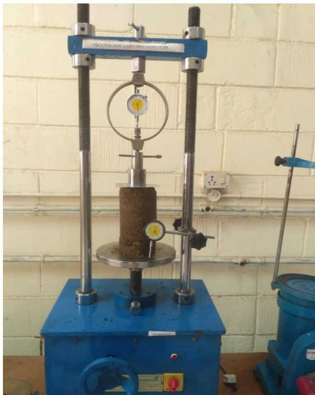
SHEAR STRENGTH OF UNREINFORCED SOIL
