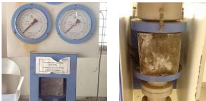
Fig -3: Compression strength of cube
