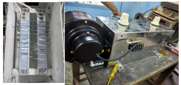
Fig.6. fringed steel & centrifugal fan used as heater
