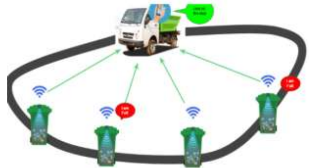
Fig -14: Truck receiving message from various bins in a particular area.
