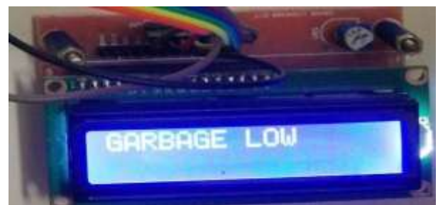
Fig -8: LCD shows the level of garbage.
