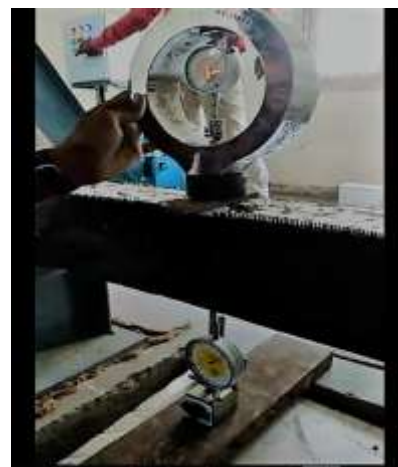
Fig-5: Testing of Retrofitted Beam Specimen
