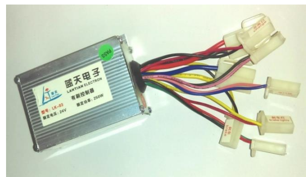
Fig -3.3: MOTOR CONTROLLER
