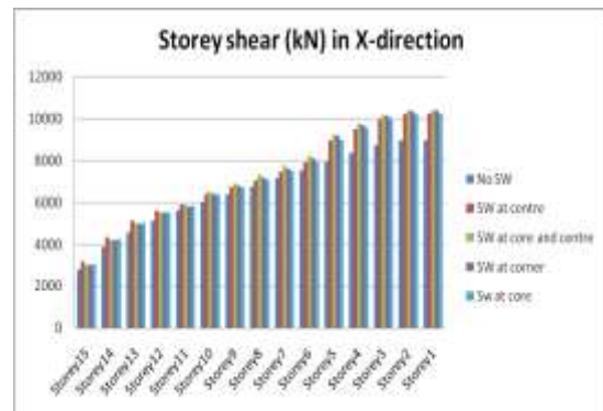
Figure-14 : Graph of storey shear of all the models with mass irregularity at 5th, 10th and 15th floor without shear wall an when shear wall is present at 4 different positions V/s storey levels in X-direction
