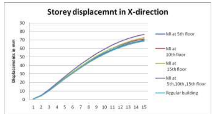
Figure-10: Graph of variation of storey displacement v/s storey levels in X-direction for 150% MI
