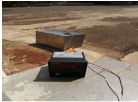
Fig -13: Conduction test for steel tank(b)
