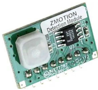
Figure 6 Passive Infrared (PIR) Sensor
