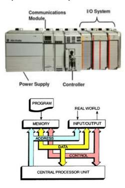
Fig -3: PLC Architecture
