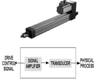
Fig -7: The Structure of an Actuator
