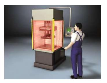
Fig -6: Model of Safety Light Curtains
