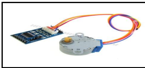
Fig -2: Stepper Motor with Drive
