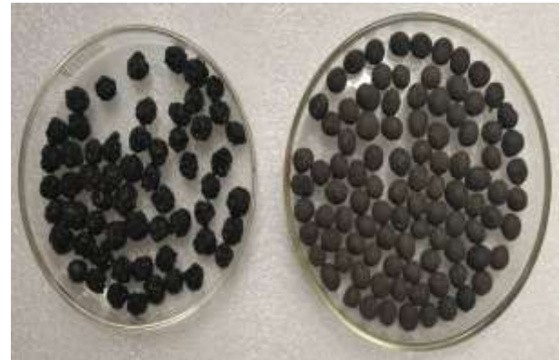
Fig -1: Rough surface and smooth surface clay beads
