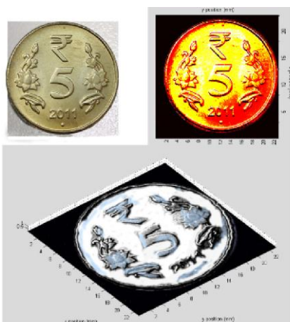
Figure 8. The construction of a 3D surface of the profile of 5 Rupee coin, using the ultrasonic scanning method.
