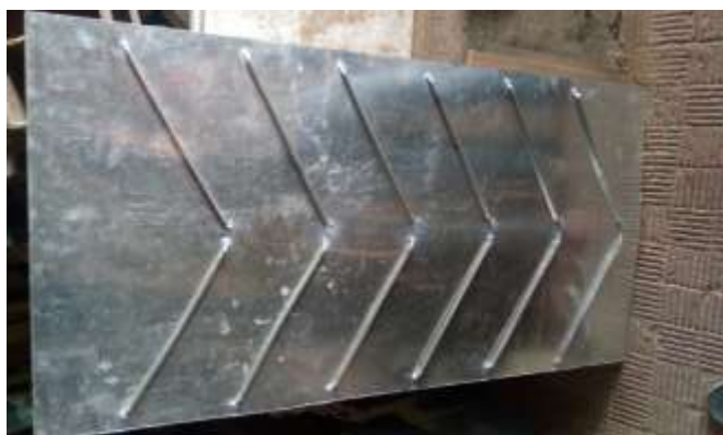
Fig -2: Arrangement of fins in V-Down Discrete Pattern
