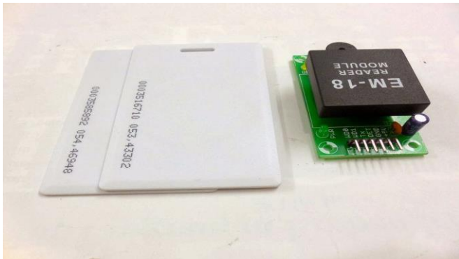
Figure 4: RFID tag and reader
