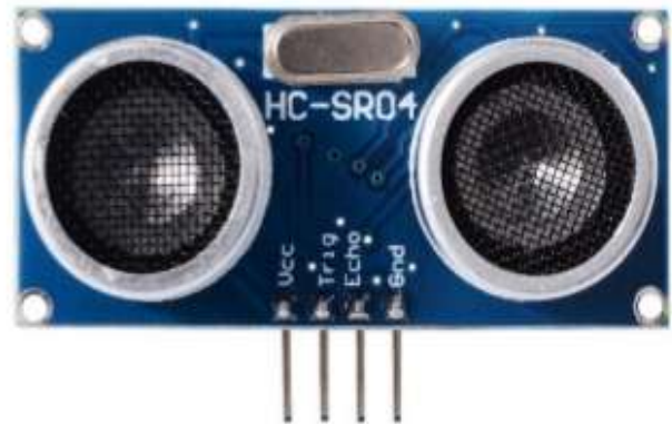
Fig 2: HC-SR04 Ultrasonic Sensor
