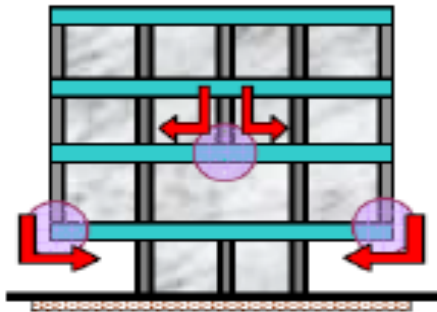
Fig -1: Floating Columns
