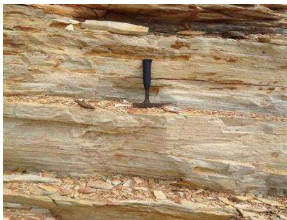
Fig 2: Photograph of quartzitic sandstone outcrop - massive with glassy texture
