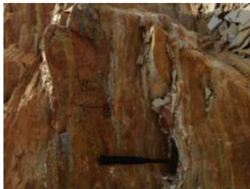
Fig 4: Photograph of sheared quartzite outcrop sections being light grey; the rock is fractured with some foliations marked by intersecting lineations
