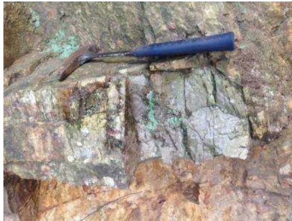
Fig -7: Photograph of recrystallised quartzite outcrop showing light grey rock with fractures
